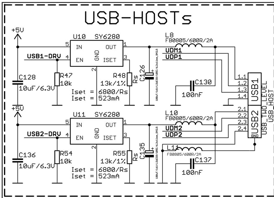
The USB\_HOST connector features two levels – called USB1 and USB2 in the schematic. The connector is situated between the USB\_OTG and the HDMI connector. Each of slots them features a Low Loss Power Distribution Switch SY6280 which protects the board in case the devices you have plugged to each level USB\_HOST try to draw more current than 523mA combined. The maximum current available on each slot of the 5V USB\_HOST is exactly 523mA.
